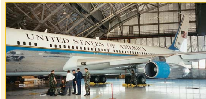
AC30-60 Platform System is used by the USAF to weigh the United States Executive fleet including Air Force One and Two.
