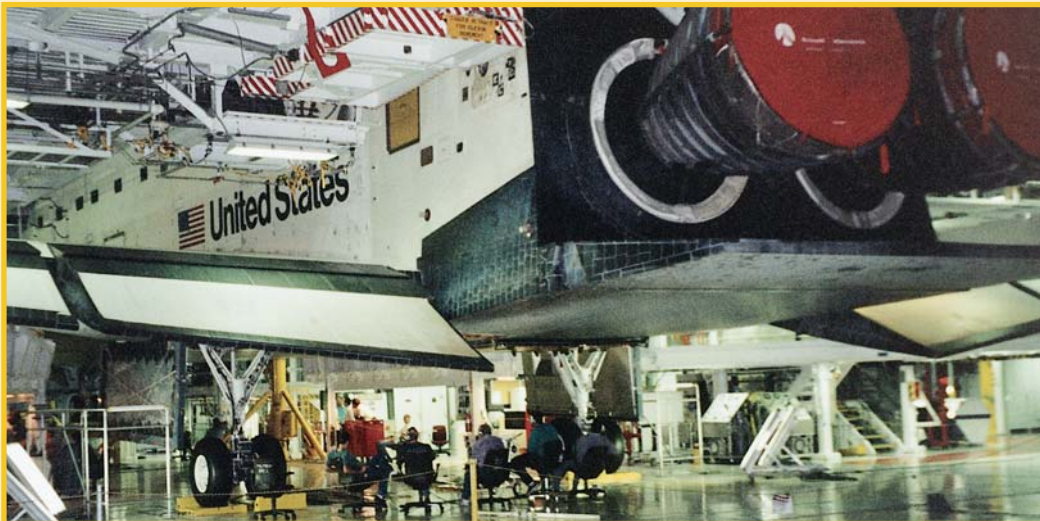
AC30-60 Platform Weighing System is used by NASA to weigh all Space Shuttle Orbiters.
